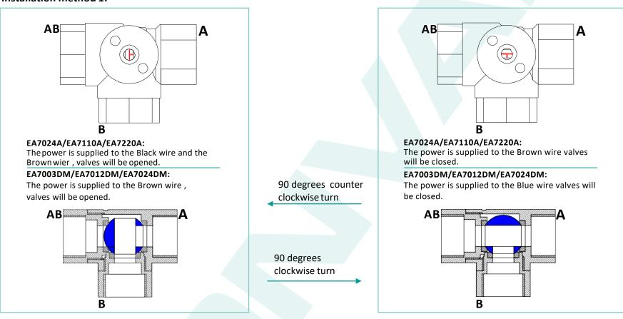
EA7220AM(A)+CBBVM315/20/25. at 90 degrees clockwise and counterclockwise turn. Core Ball is "T" mode.
