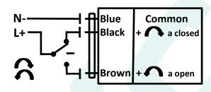
Valve (ON) : Brown wire Valve (OFF) : Black wire Com(N) : Blue wire
