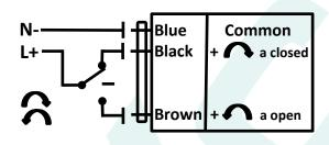
Valve (ON) : Brown wire Valve (OFF) : Black wire Com(N) : Blue wire
