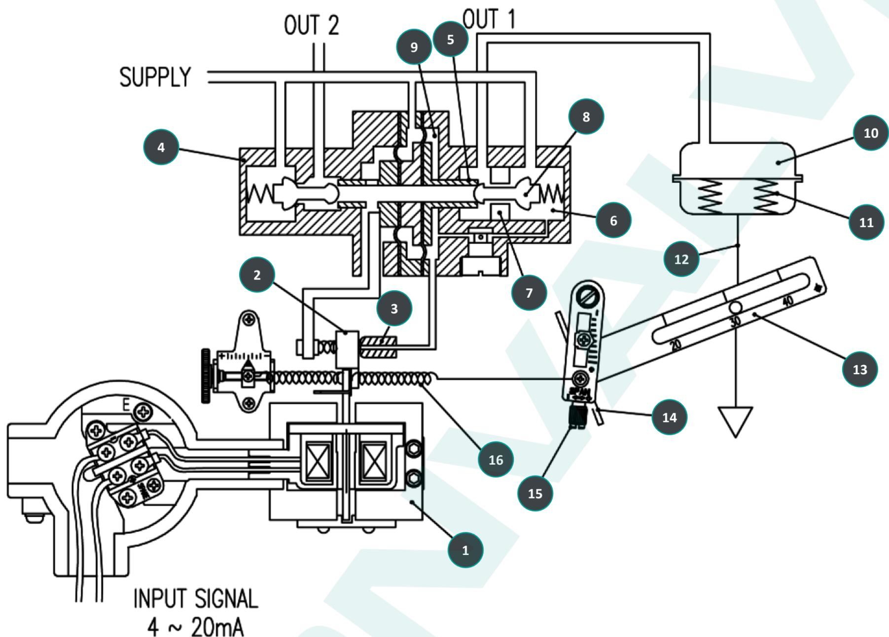
When an INPUT SIGNAL is supplied to the positioner to open the valve, power is generated from the torque motor and pushes the flapper (2) to the opposite side of the nozzle (3). This widens the gap between the nozzle (3) and the flapper (2), causing the air inside the chamber (9) to exhaust through the nozzle (3) from the inner part of the pilot (4) to the left of the spool (5).
