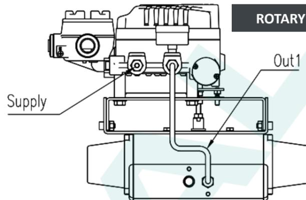
Based on the provided diagrams, it is crucial to ascertain whether the valve operates in a "Reverse Acting" or "Direct Acting" manner. Subsequently, it is necessary to establish the appropriate connections between the positioner's OUT1 port and the actuator's port accordingly. If required, the assembly position of the Span (Linear) and Cam (Rotary) components may be adjusted for optimal performance.
