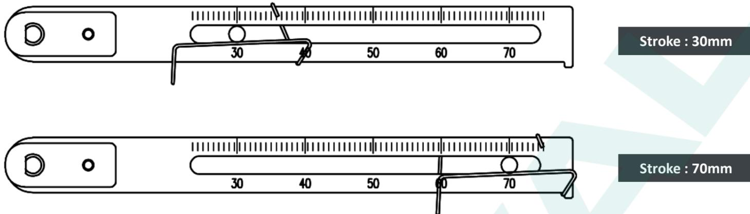
8. Once the positioner is installed, proceed to operate the valve, moving it from 0% to 100% stroke using direct air supplied to the actuator. At both extremes of the stroke (0% and 100%), carefully observe the linear lever stopper's position in relation to the stopping bosses on the backside of the positioner. Ensure that there is no contact between the linear lever stopper and the stopping bosses.
