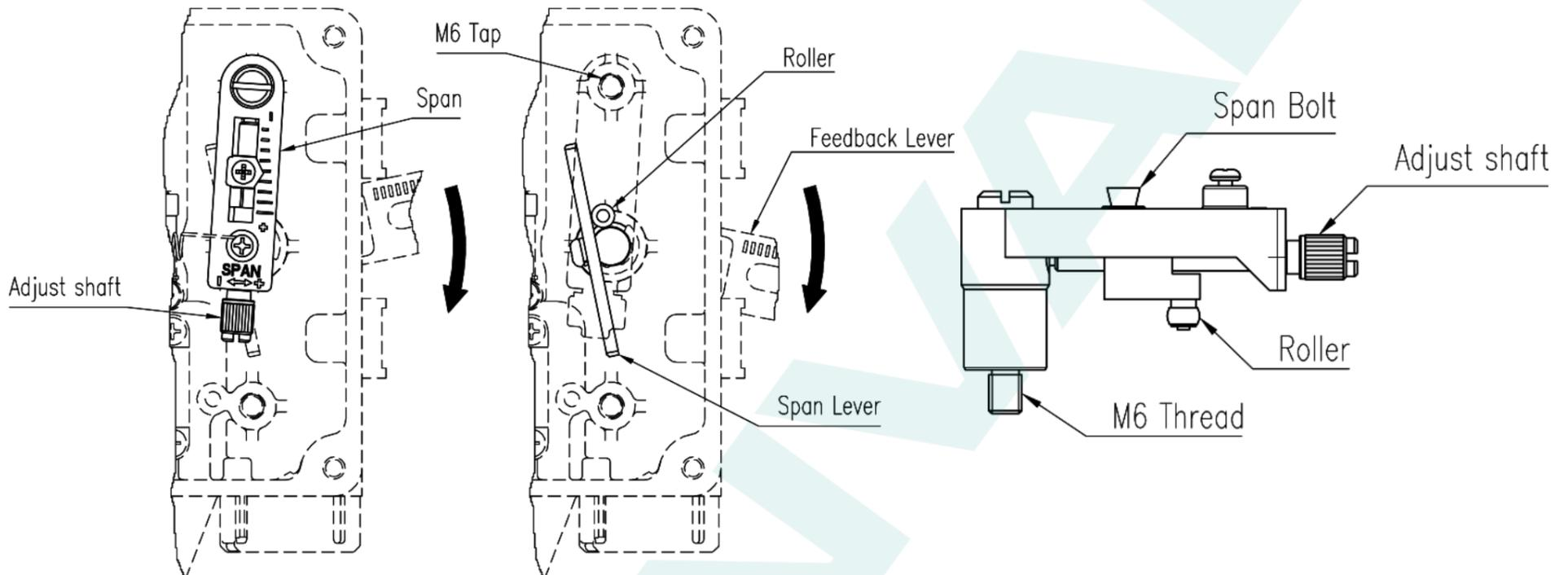
2. If the actuator axis moves up when the input signal is increased, follow the assembly instructions for the "Span" component as shown in the figure below:
