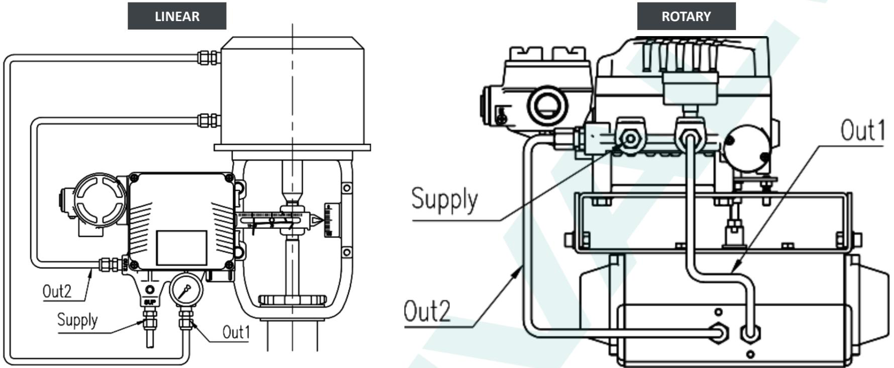
Based on the provided diagram, analyze the valve's behavior to determine if it is "Reverse Acting" or "Direct Acting."
