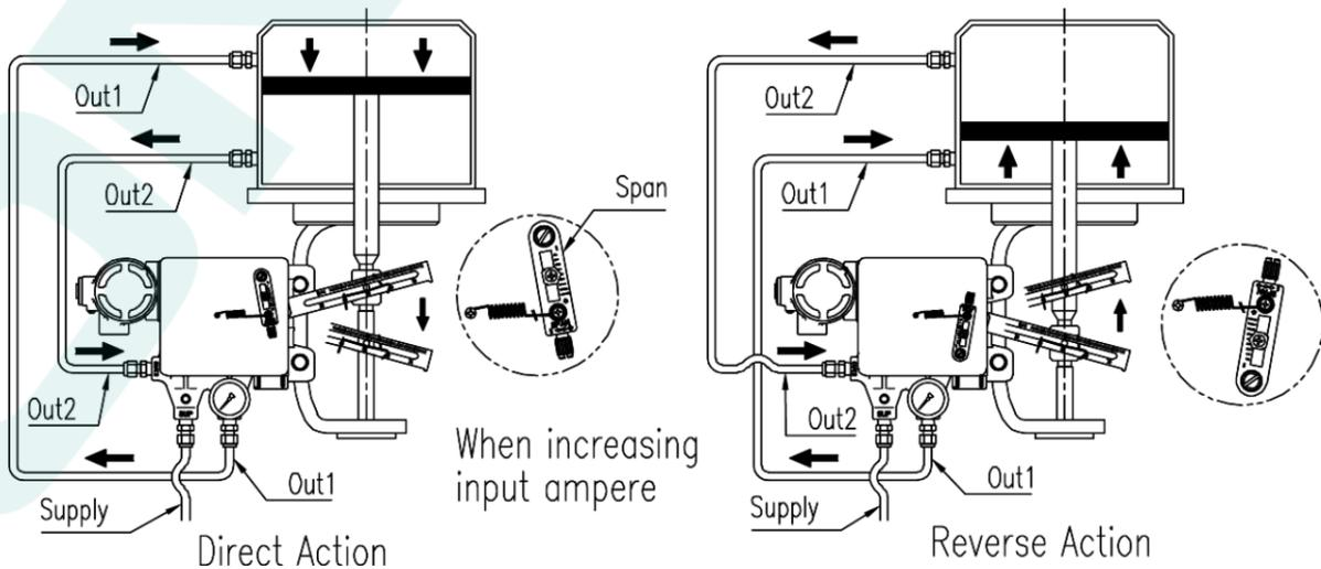
**SETTING DIRECTIONS OF PIPING AND CAM FOR ROTARY DOUBLE ACTUATOR**
