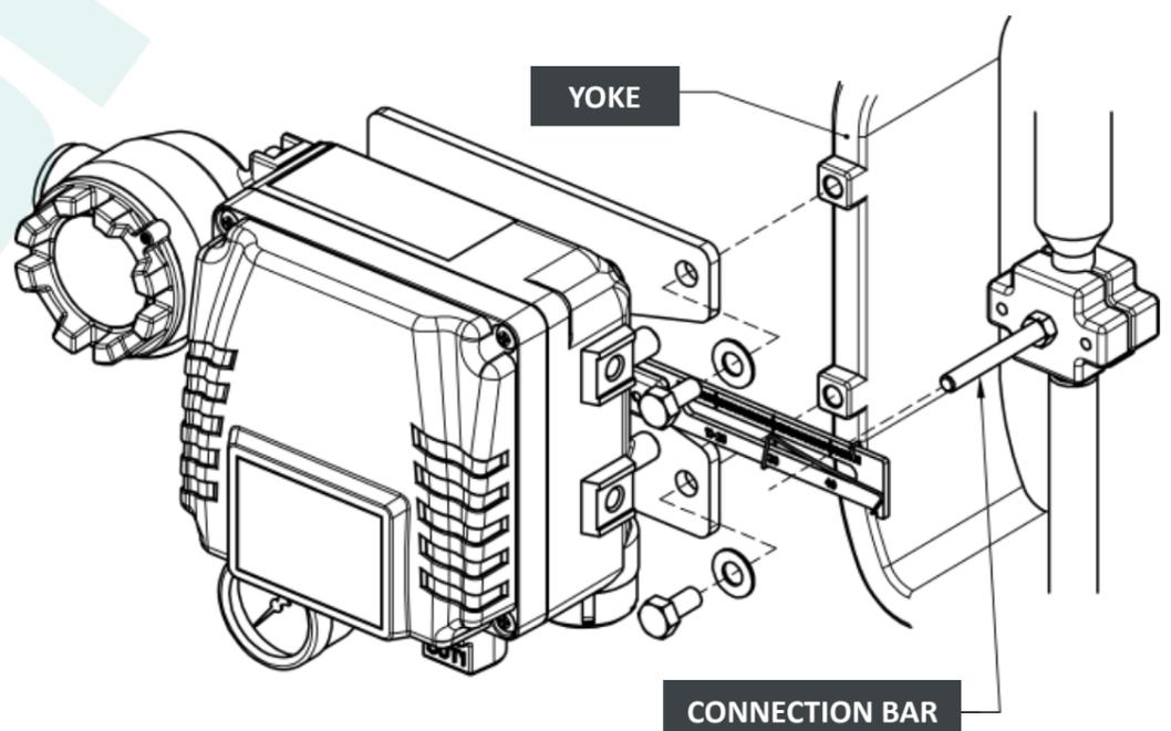
ATTACHING THE BRACKET TO ACTUATOR YOKE
