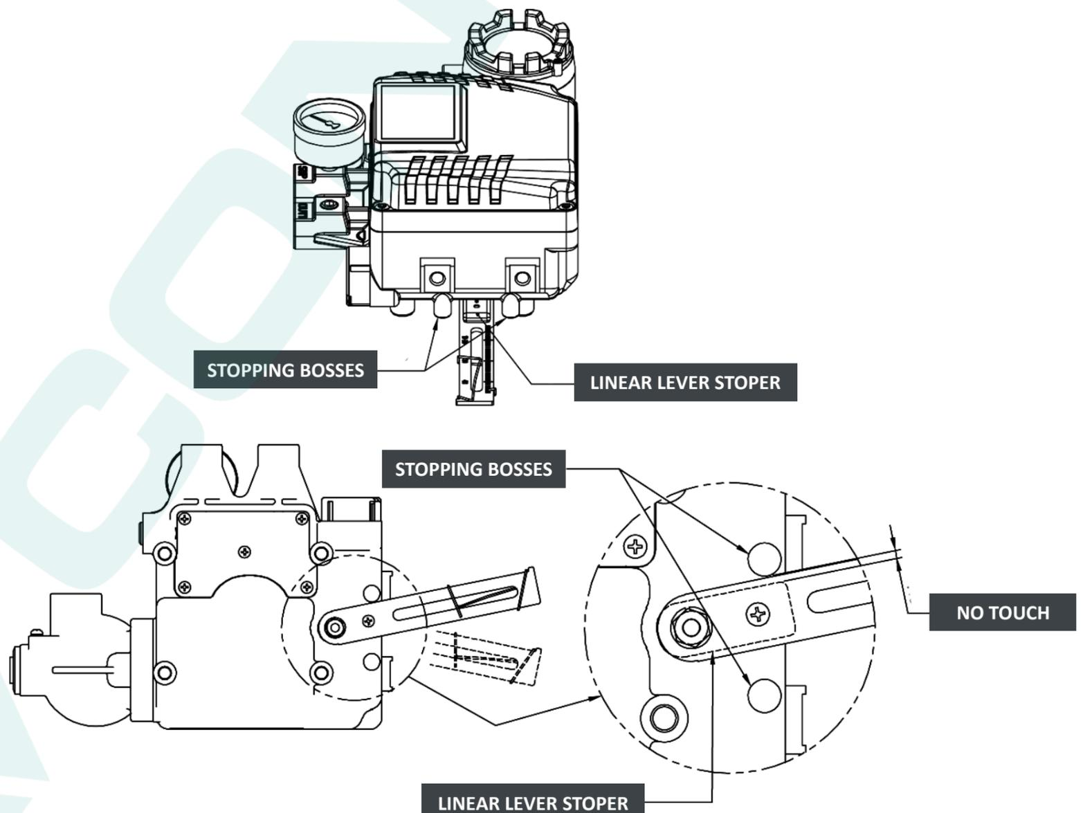
9. Following the installation, proceed to securely tighten all bolts or nuts on both the bracket and the connection bar. Ensuring proper fastening of these components is vital for the stability and reliable performance of the positioner and the associated linear motion valve.
