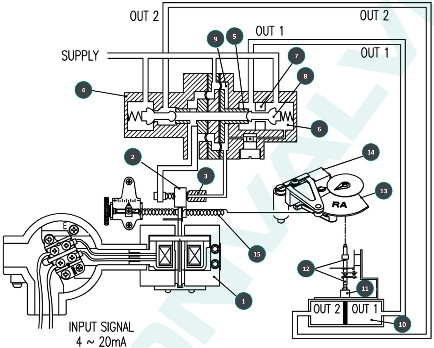
When an input signal is supplied to the positioner to open the valve, power is generated from the torque motor (1), which pushes the flapper (2) to the opposite side of the nozzle (3). As a result, the gap between the nozzle (3) and the flapper (2) widens, and air inside the chamber (9) from the inner part of the pilot (4), left to the spool (5), is exhausted through the nozzle (3).
